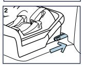
3 Pull the base back to ensure both lower connectors are engaged.
